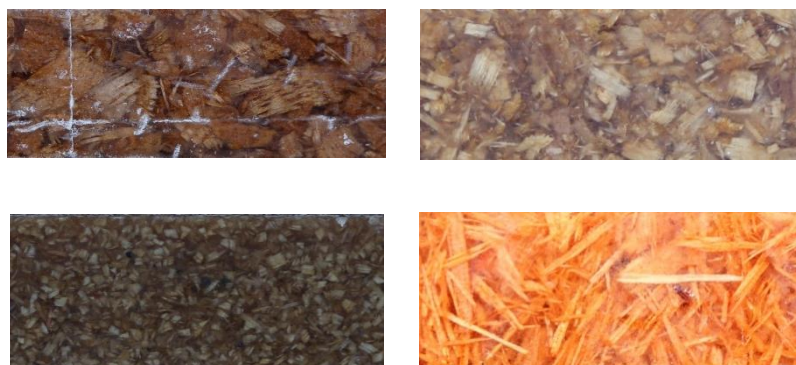
Figure 2. Macro Structure of wood flour (WF) in square dimensions (very coarse, coarse, and medium) as well as the length and rough dimensions
